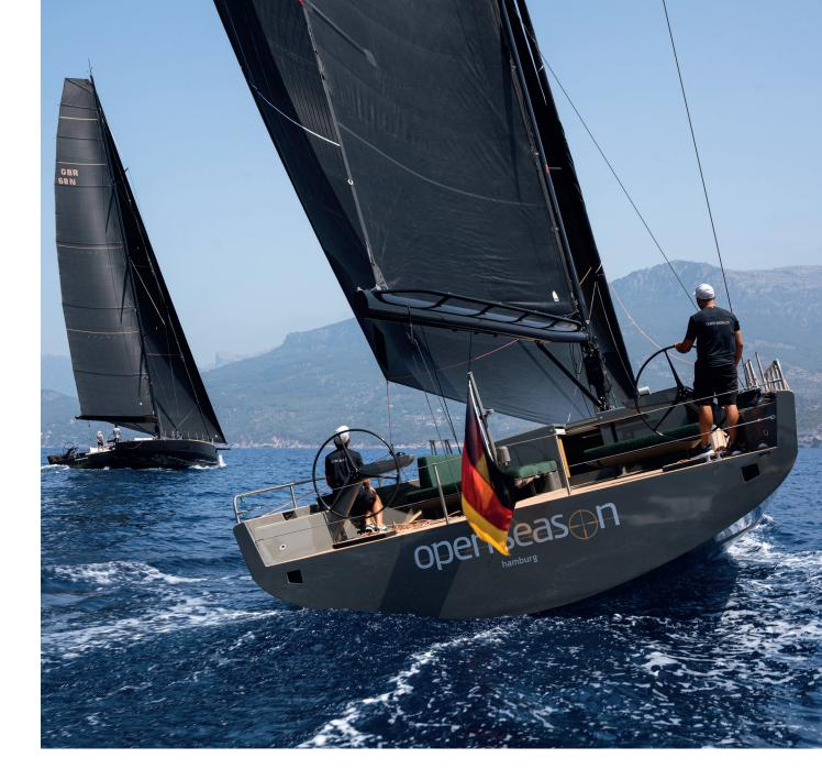
It is clear that the owner of *Open Season*, a seasoned racer on the Mediterranean circuit, has a far greater focus on pure performance. As such, the boat has been built in pure carbon with the flax reinforcement dispensed with. The deck is pre-preg Nomex to further keep the weight down. This has made it significantly lighter, with the new boat weighing in at 20,600 tonnes as compared to the 22,800 tonnes of hull number one. Beyond that though, there are other significant
